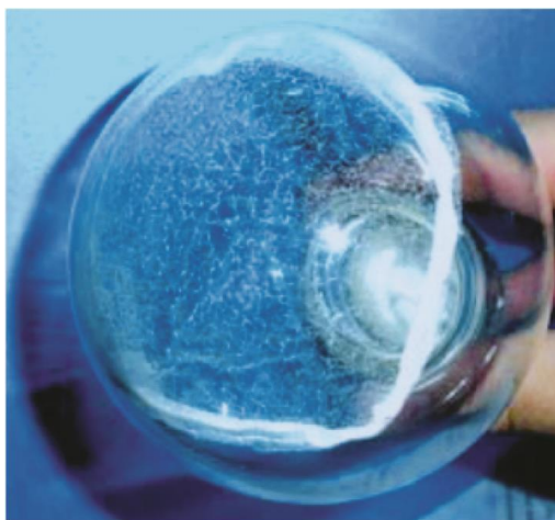
Fig. 30. This image shows the solid residue left in a flask after freeze-drying 250 ml of water iteratively treated with Nafion.
